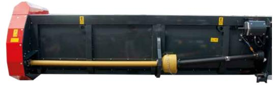
In its basic configuration, HELIANTHUS PRO has an independent from the combine harvester adjustment angle during the work in the field. This feature prevents seed spilling from the dividers.
