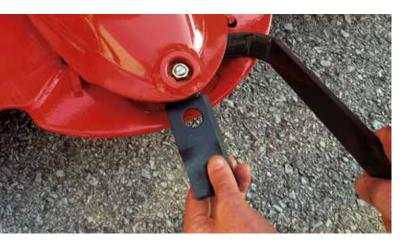
Quick-change knives dramatically reduce replacement time without the use of tools. Cutting discs are made to have a remarkably close proximity of knives and provide a perfect cut even with packed and wet product.
