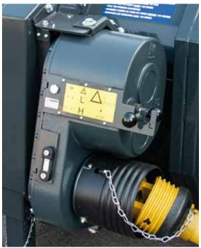
Continuous feeding: thanks to the integrated gearbox on all headers, it is possible to change the auger speed and cutting length of the harvest at the same time with a simple gear shift.
